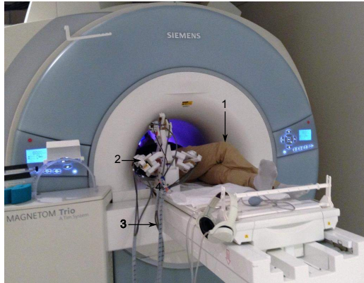
Fig. 9. MR-SoftWrist location during fMRI. 1) Subject, 2) MR-SoftWrist, and 3) encoder and power lines.
