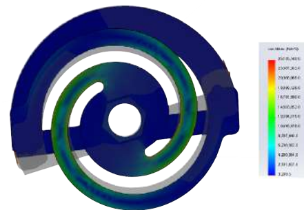
Fig. 5. FEM simulation of Delrin spring, with inner annulus blocked and loading torque applied through the capstan arch. The two outer ends of the double spiral are rigidly connected through the capstan arch. The predicted stiffness equals 0.175 N m deg -1 , and the resulting maximum von Mises stress is 2.5 times smaller than Delrin yield stress (62MPa).
